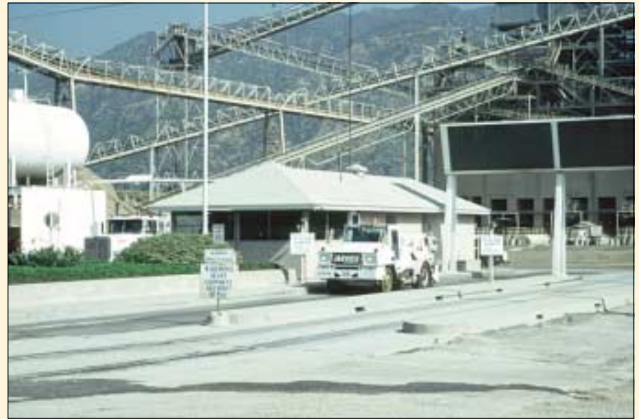
Figure 14. Dust control techniques include the use of water trucks and sweepers on haul.
